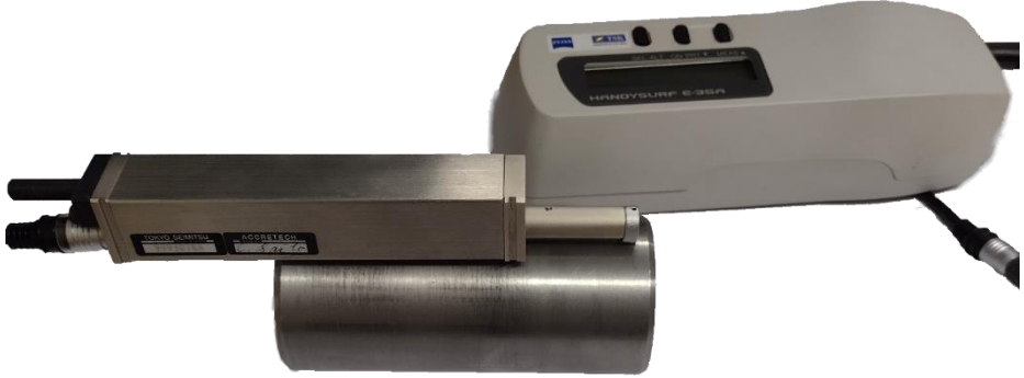
Fig. 1. Measurement of surface roughness using the roughness tester.
