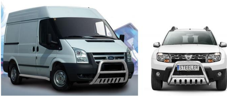
Fig. 2. The front protective stainless steel frames are now often replaced by composite frames.
