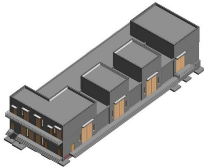
Fig. 2. Substation Building 3D Model
