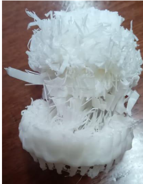
Figure 5 Failed PLA Filament 3D Printed Oral Mannequin
