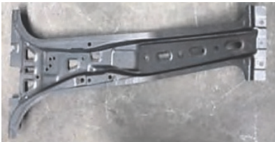
Fig. 1. Physical photo of B-pillar.
