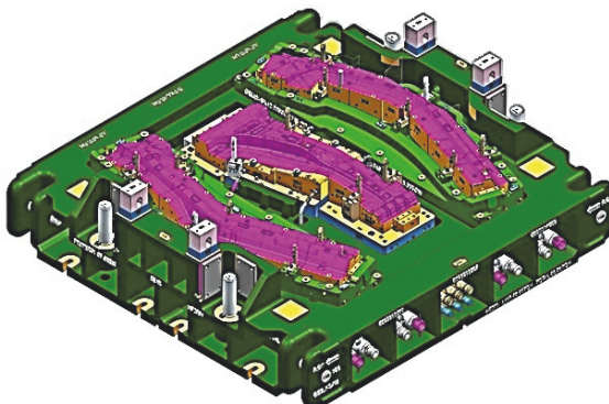
Fig. 10. Mold diagram for hot stamped products with multiple parts in one die
