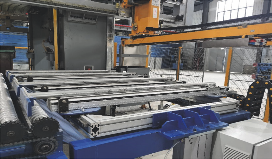
Fig. 6. Digital servo blocking system at the discharge end of the heating furnace
