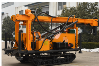
Fig. 1. Water Well Drilling Rig
