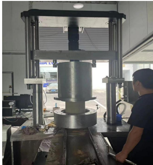
Fig. 3. The sample is being loaded into the pressure chamber
