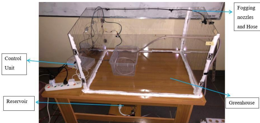
Fig. 3. Overall setup of the irrigation system
