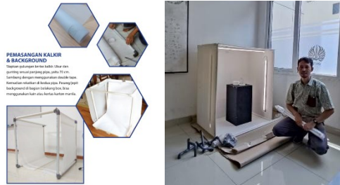
Fig. 3. Portable photo box assembly process.
