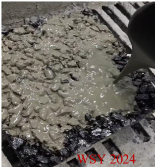
Fig. 4. Perfusing cement grout
