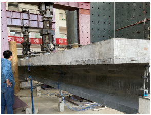
Fig. 3. Field loading diagram of test beam
