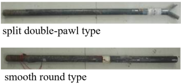
Fig. 1. anchor bolts and anchorage concrete
