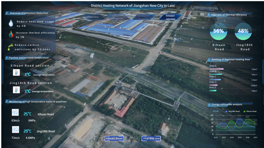
Fig. 4. Digital Twin Carbon Emission Monitoring Module for District Heating Networks
