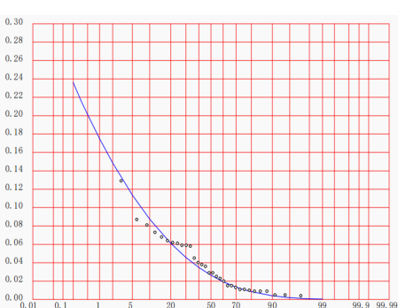
Fig. 2. Frequency diagram of increased value of unit water consumption of textile industry
