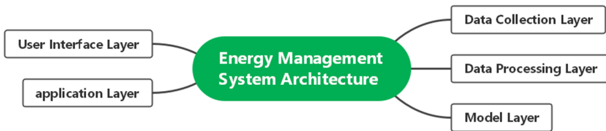
Fig. 2. smart building architecture based on digital twin
