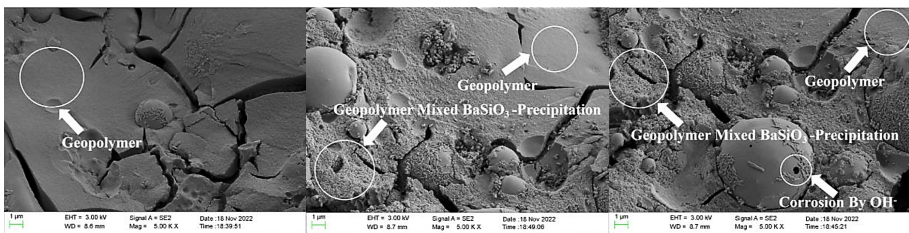
Fig. 4. Micro- morphology of F8-4, B1. 5 and B2 at 28 d age
