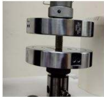
Fig. 10. Kelvin truss lattice structured Compression test specimen and Instron 3369
