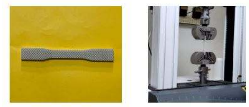
Fig. 5. Iso truss lattice structured tensile specimen and Instron 3369 UTM
