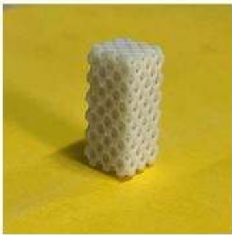
Fig. 10. Kelvin truss lattice structured Compression test specimen and Instron 3369
