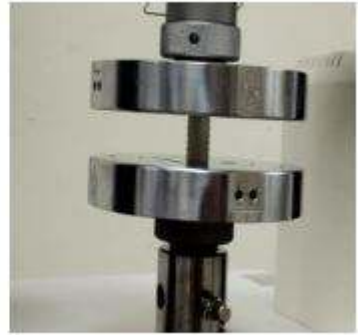
Fig. 9. Iso truss lattice structured Compression test specimen and Instron 3369 UTM
