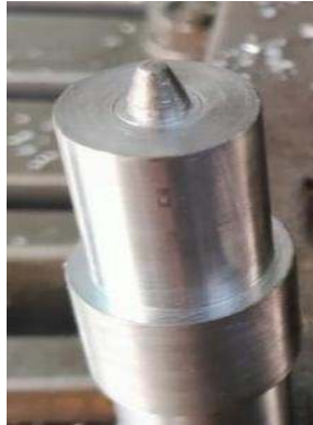
Fig. 3. Tapered Cylindrical Tool Profile
