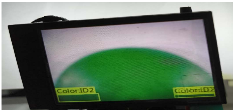
Fig. 4. Green Color is coded as ID:2 is identified by the huskylens.
