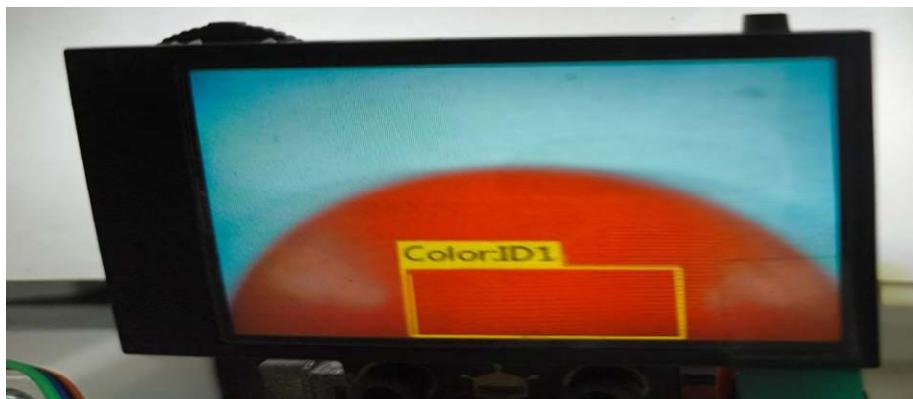
Fig. 3. Red Colour is coded as ID:1 is identified by the huskylens.
