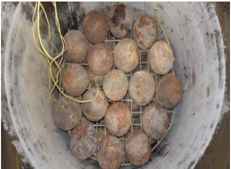
Fig. 3. PCM capsules arrangement in the TES tank
