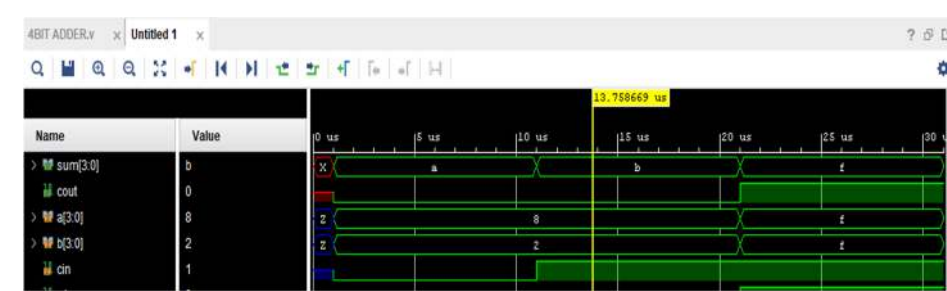
Fig. 5. Waveform of Conventional Carry Select Adder
