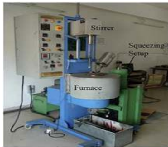
Fig. 1. Efficient setup for stir casting in MMC manufacturing.
