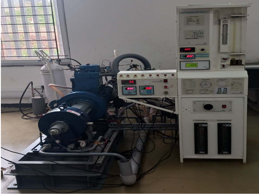
Fig. 1. VCR diesel engine experimental setup
