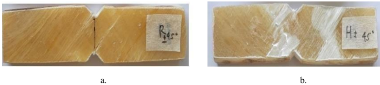
Fig. 7. Composite specimens with fiber directions of 45^\circ : a. ramie/epoxy 45^\circ , b. hybrid ramie-E-glass/epoxy 45^\circ
