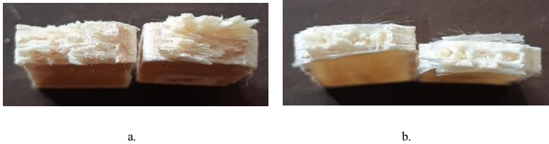
Fig. 9 Transverse position of failure mode that occurred in the composite specimens: a. ramie/epoxy, b. hybrid ramie-E-glass
