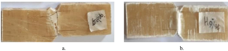
Fig. 8. Composite specimens with fiber directions of (0^\circ, 90^\circ)_s : a. ramie/epoxy (0^\circ, 90^\circ)_s , b. hybrid ramie-E- glass/epoxy (0^\circ, 90^\circ)_s
