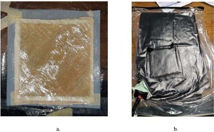
Fig 2. Lamination method of composite specimens: a. hand lay-up, b. vacuum bagging
