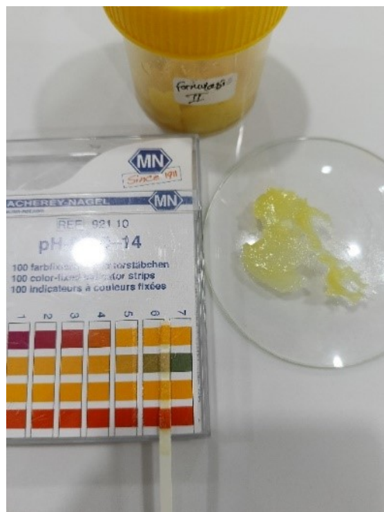
Fig. 2. Formulation II pH Test Results
