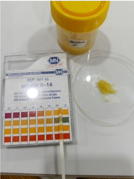
Fig. 4. Formulation IV pH Test Results
