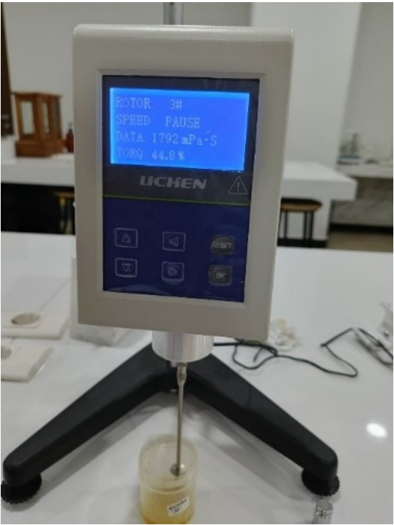
Fig. 7. Formulation 4: Not measurable (over), indicating viscosity is too high for topical application and requires adjustment.
