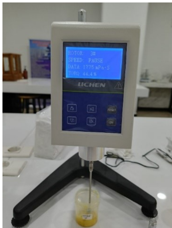
Fig. 6. Formulation 3: Highest viscosity of 1792 mPa.s and torque of 44.8%, indicating good stability for optimal dispersion.
