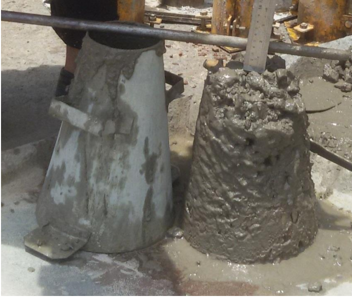
Fig. 2. Slump test of fresh concrete
