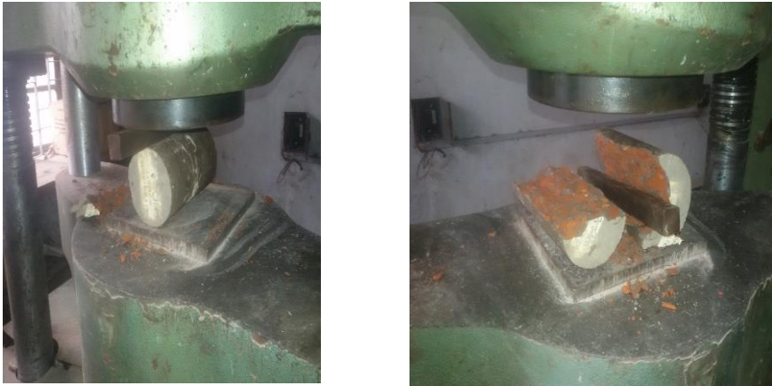
Fig. 3. Compressive strength test during loading and specimen after failure
