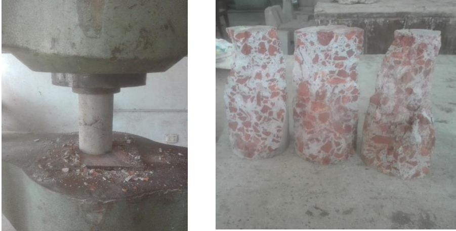
Fig. 3. Compressive strength test during loading and specimen after failure
