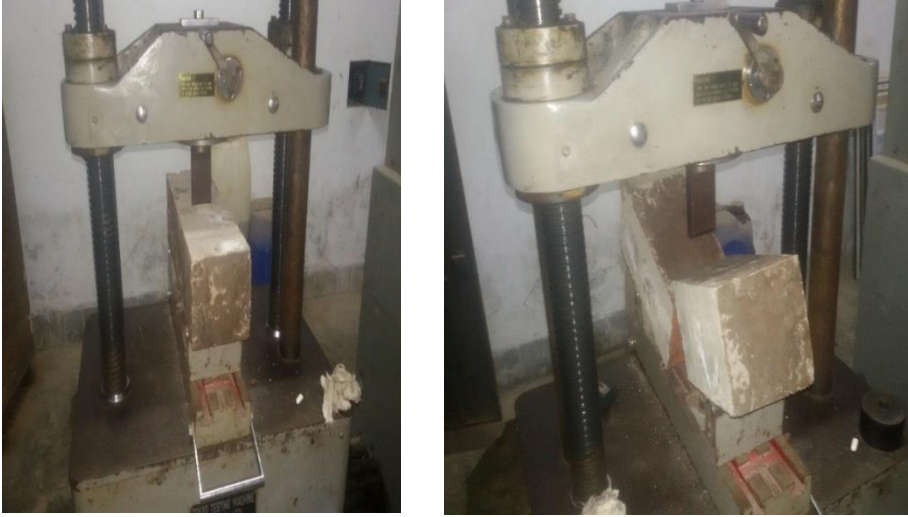
Fig. 5. Flexural strength test during loading and specimen after failure
