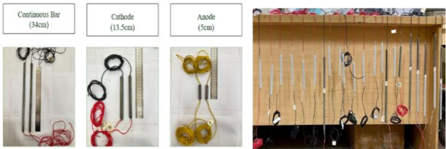
Fig. 2. The connection of the coated steel bars with wires.
