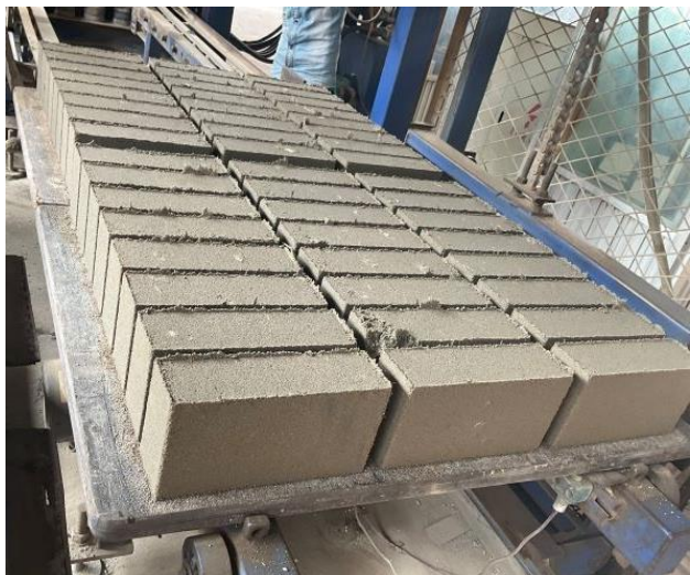
Fig. 1. Concrete Blocks During Production: Freshly Moulded Units Prior to Curing
