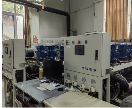
Fig. 2. Physical photos of flue gas heat recovery test-bed.
