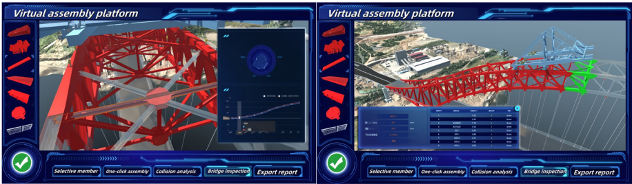
Fig. 10. Installation of segments H21a and X9a and segment analysis prediction
