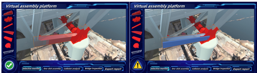
Fig. 7. Assembly correct and collision error
