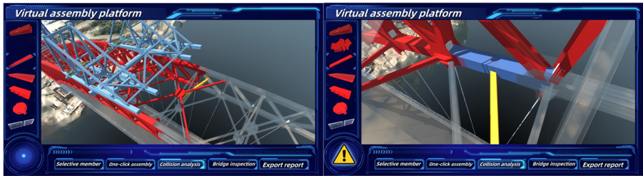
Fig. 8. Lifting simulation and collision visualization
