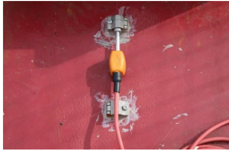
Fig. 5. Composite strain acquisition sensor
