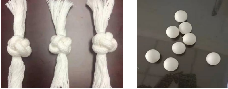
Fig. 1. Core and shell of the rope knot temporary blockage ball.
