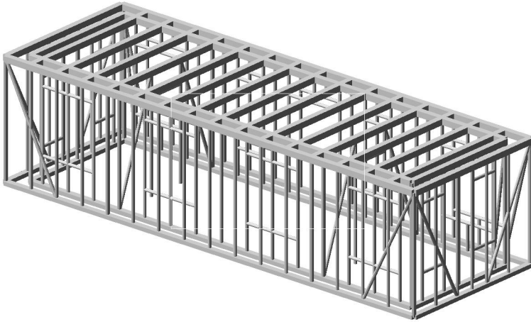
Figure 3. General view of the simulated system for options of problems No. 1, No. 2, and No. 3 (elements of the foundation, filling of the “sinch” frame and elements of the ceiling are not shown).
