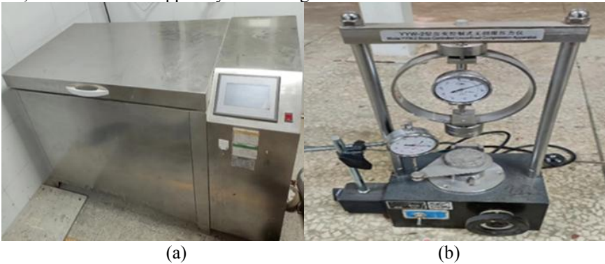
Fig.2. (a) Freeze-thaw test machine; (b) Strain-controlled unconfined pressure gauge.
