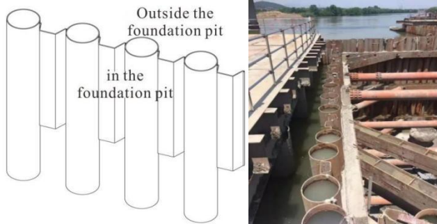
Fig. 3. Schematic diagram of vertical enclosure structure for PC construction method piles (a. schematic diagram of enclosure structure; b. on-site construction diagram)
