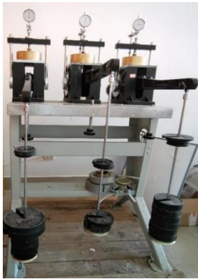
Fig. 2. Model WG consolidation meter(photographed by the author)
