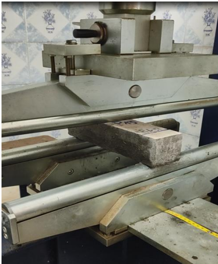
Fig. 3. Flexural strength tests.
