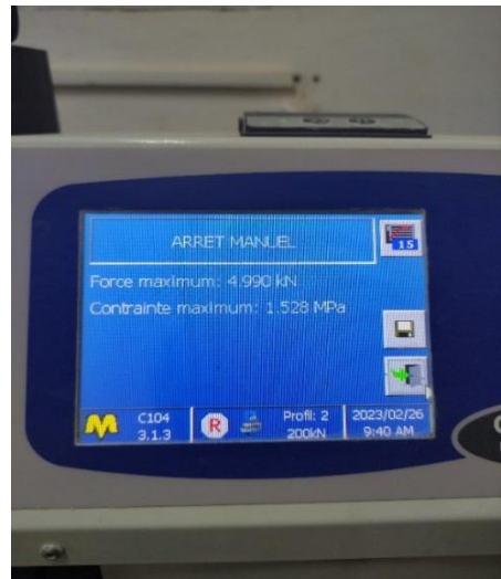
Fig. 3. Flexural strength tests.
