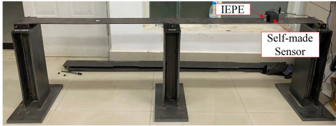
Fig. 7. Deployment diagram of IEPE sensor and self-made sensor
