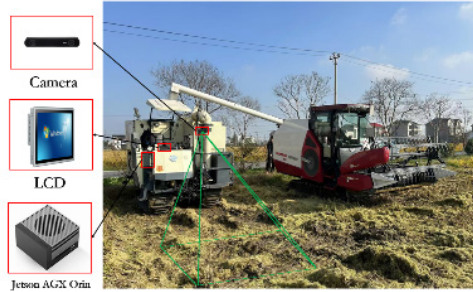
Fig. 1. Onboard Vision System of the Grain truck
