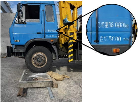
Fig. 11. Field load-bearing capacity test of concrete slab after renovation.
