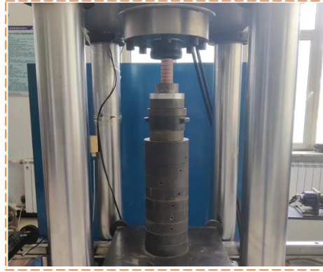
Fig. 3. TAW-2000 rigid pressure testing machine
