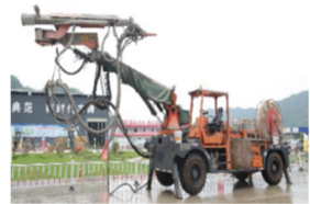
(c) Concrete wet spray truck
