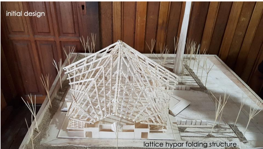
Fig. 5. Physical model of the mosque using hypar + folding structure
