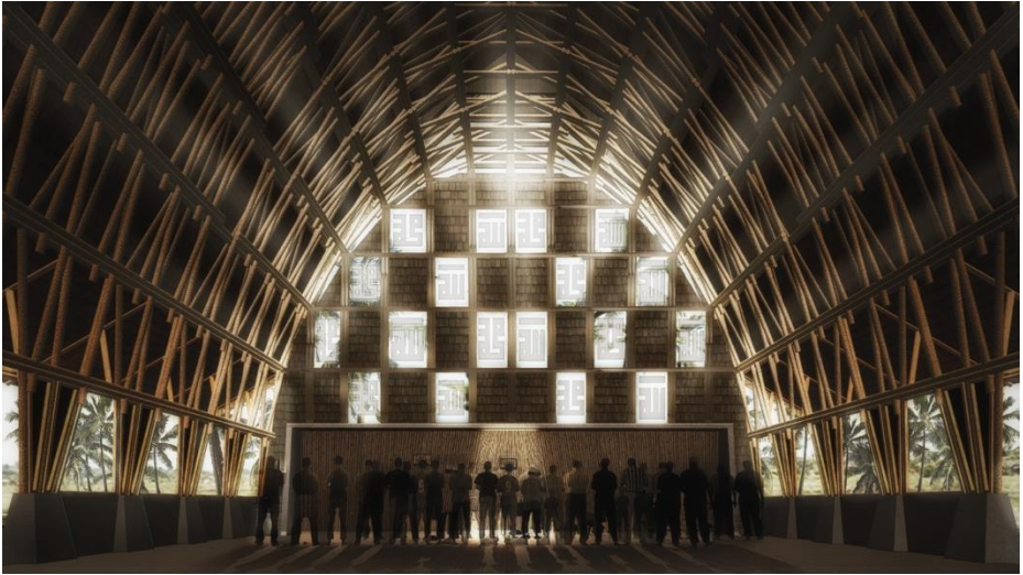
Fig. 3. The interior of the mosque showcases the grandeur of the layered bamboo structure
