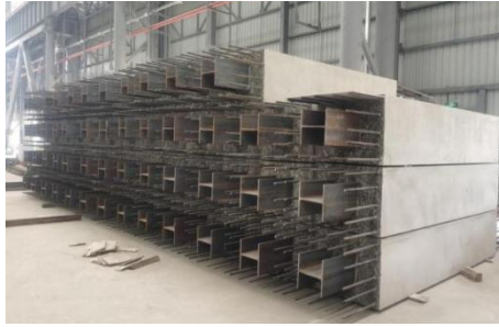
Fig. 10. Stacking of Prefabricated Columns
