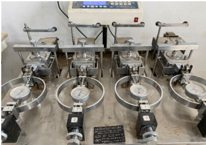
Fig. 4. ZJ strain controlled direct shear instrument.
