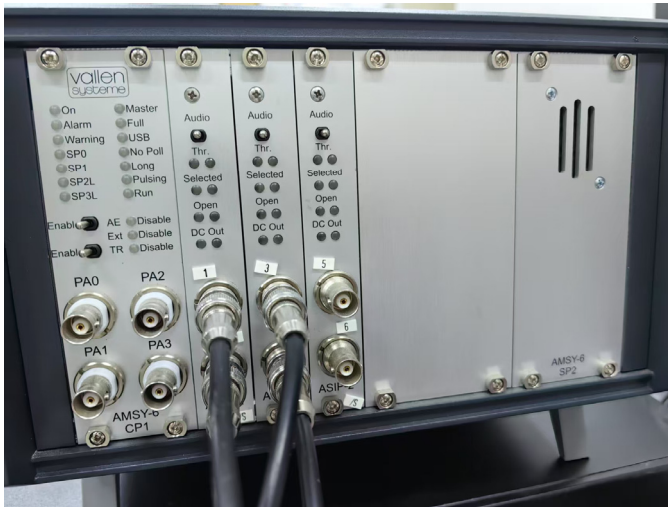
Fig. 5. Acoustic emission monitoring equipment.
