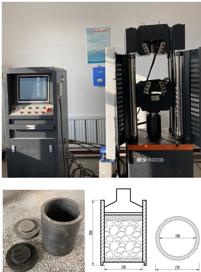
Fig. 1. Electrohydraulic servo universal testing machine and compression device diagram.
