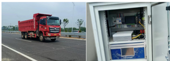
Fig. 2. Load information acquisition system
