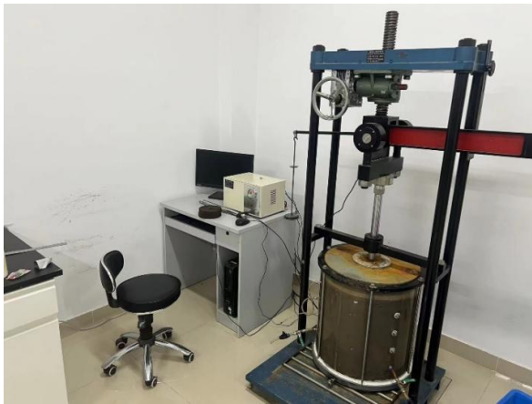
Fig. 4. Testing device for three-dimensional drainage body consolidation test.
